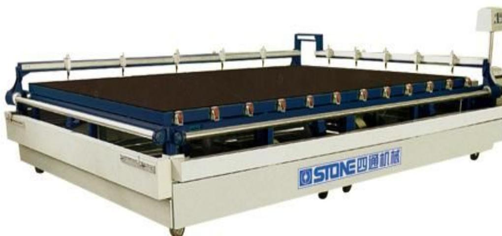
The semi-automatic, dual-bridge precision cutting table is improved by using gear-drive equipment
