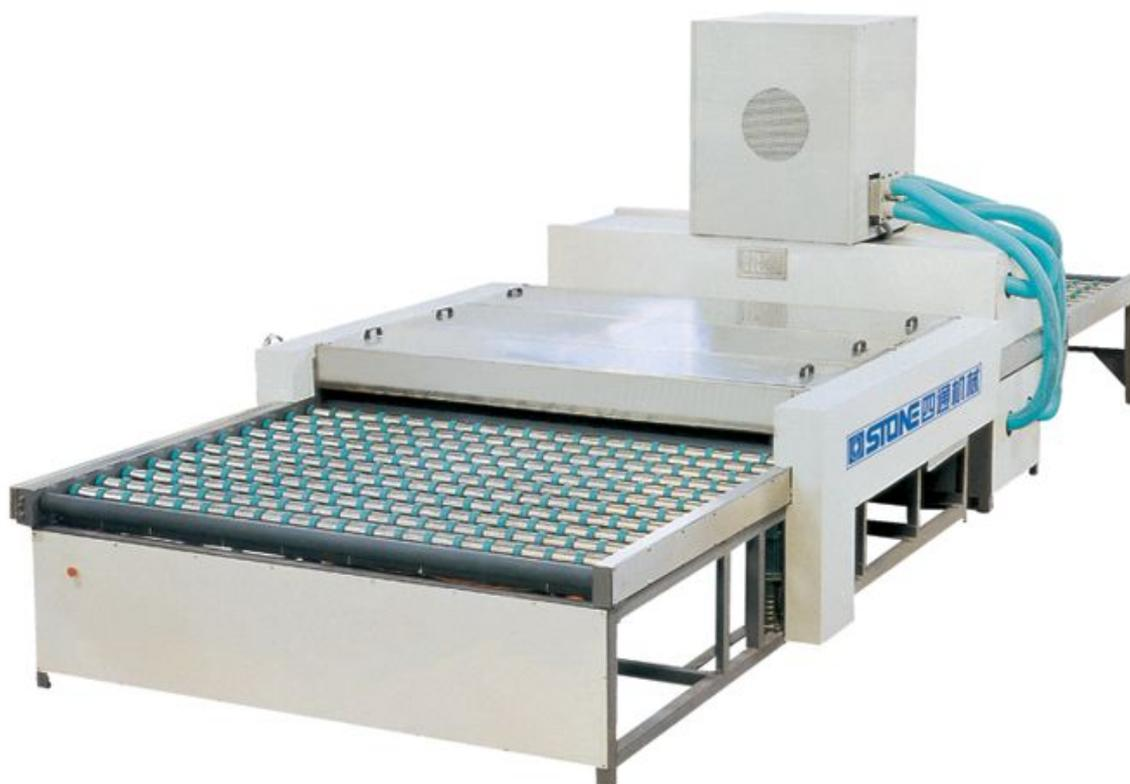
Automatic clean and dry flat glass with the thickness of 3-19mm. Using 3 pairs of brushes to wash and air knives which supply strong cold wind to dry the glass. Especially suitable for clean the glass before coated, making mirror, laminating and tempering.
