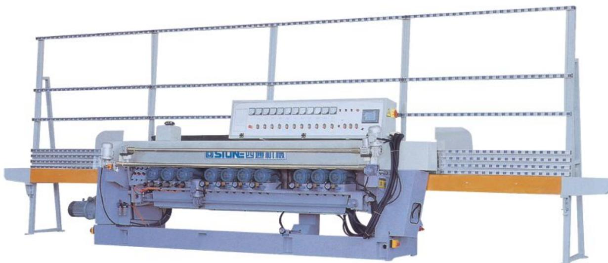
Controlled by PLC with automatic and manual operation modes, adjust speed with stepless regulator; 11 motors rough grinding, fine grinding, bottom edging and pneumatic polishing can be finished at one time. Processed bottom edge is round shape, the front conveyor has up-and down adjusting system, can adjust according to the size of glass.
