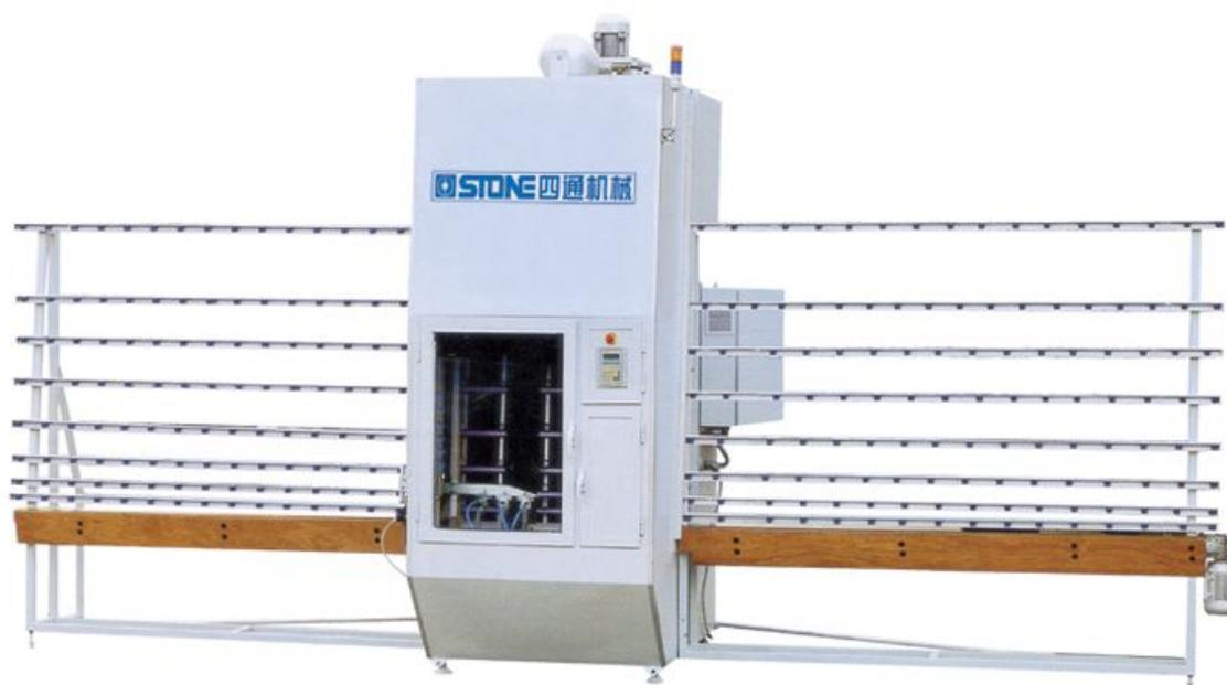
Use air-compressor to drive sand into the sanding gun processing Varieties of patterns on the surface of glass, ceramic and plastic.
