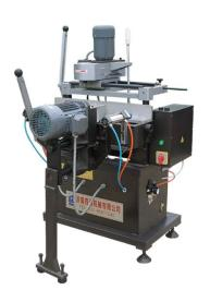
Lock-hole Groove Processing Machine is a special machine used for processing transmission device installing holes and grooves for plastic doors and windows. It consists of long horizontal holes. One time clamping can achieve 2 working procedures, which ensures the precise position between holes and grooves efficiently.
