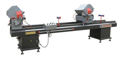
This machine is used for processing the aluminum and plastic profiles at angles of -45 to 90 to 45 degree. The Two heads can work individually, simultaneously and combinatively. It has the features of simple operation, stability and high efficiency.
