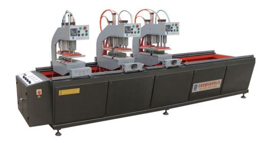
Three-head Welding Machine is a special machine for processing plastic doors and windows. It can weld doors and windows in many figures and the combination. PLC and pneumatic driving systems are used to achieve processing range. The 3 heads can work individually, simultaneously. **Main parameter:**
