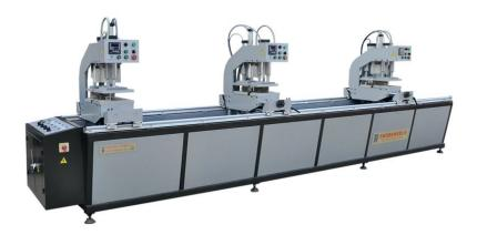
Three-head Welding Machine is a special machine for processing plastic doors and windows. It can weld doors and windows in many figures and the combination. PLC and pneumatic driving
