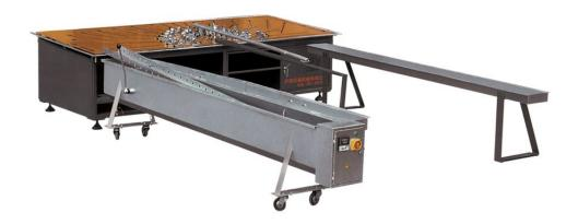
Arc Window Machine is a special machine for processing are windows. It includes the working table, the heating device and the shape-forming bands. The media oil is heated by electricity, and the profile is heated in the media oil. The semi-circle with the diameters from 500mm to 1800mm can be processed. With different shape-forming bands, it can process various profiles. It has features of reliability, safety and high efficiency.
