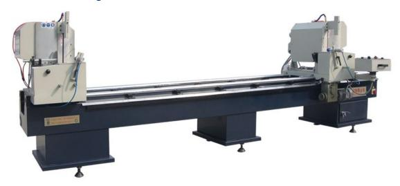
Double-head Cutting Saw is used to process the aluminum and plastic profiles at angles of -45 to 90 to 45. Pneumatic driving system and linear feeding ensures the stable operation. The movement of the two heads is driven by the motor. The machine has the advantages of good rigidity, reliable operation, high accuracy, large processing range and high efficiency.
