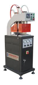
Single head welding machine for PVC window frame is the main assistant machine for Plastic Door and Window, it can weld with variable angle ranging from 30 to 180 degree.
