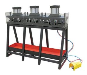
It is a specially designed for American style profile. It is pneumatic control and can drill different profiles through changing the die .lt features high reliability, easy operation and high precision etc.
